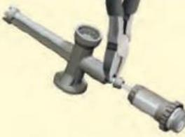
C. Remove/Install Rod End
